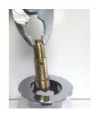
Using a pair of pliers, grip the flat end of the plunger and unscrew the plunger from the waste body.
