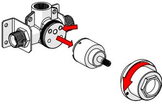
**5. Remove cartridge nut and check cartridge**
