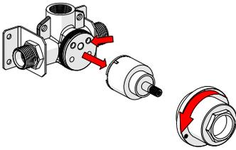
**5. Remove cartridge nut and check cartridge**
