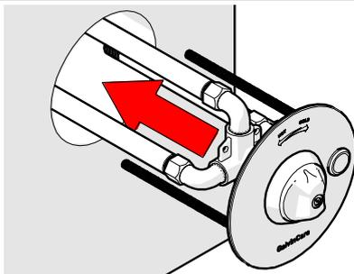
2. Apply silicon sealant to the lip on the faceplate to seal faceplate to the wall.
