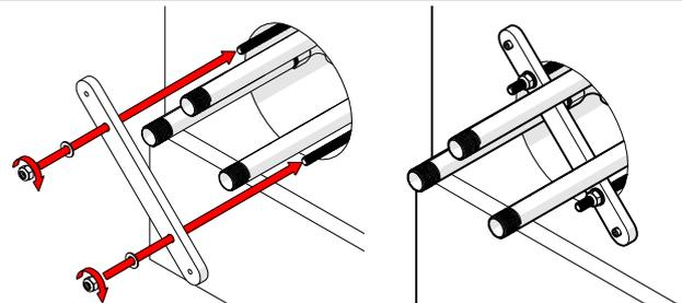
4. Secure the unit using the supplied back brackets, washers and nuts (as shown).
