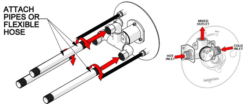
1. Fit hot, cold and outlet water pipes to the shower unit. (Elbows not supplied).
