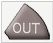
**DELAY OUT TIME:** This button allows modifying the flushing stop time after the user moves away from the sensor range. A delay out time close to 0 will save more water. An increased delay out time will make the user experience more comfortable.
