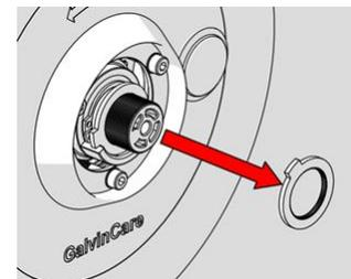
3. Remove the upper brass ring. Make sure the control rod doesn't rotate during the next steps.
