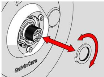
4. Remove the lower brass ring (temperature setting ring) and rotate the brass ring clockwise to increase temperature or anti-clockwise to decrease. Refit to spline in new position.
